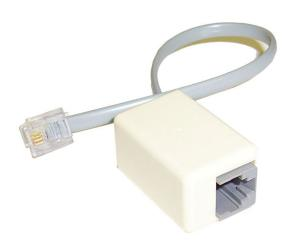
The M-150 filters are single pair, in-line filters designed to attenuate RFI up to -57 dB on analog lines from 75 kHz to 150 MHz. The filters require no external grounding and are balanced to 600 ohms with an off-hook insertion loss of less than 0.1 dB at 1004 Hz, thus ideal for telephony applications such as with telephones, fax machines and analog PC modems.
